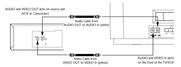
Make the connections shown above, using audio and video cables (not supplied). Connect the source unit (VCR or Camcorder) to a power source after connections are made.
